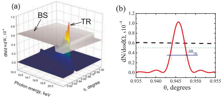
Fig. 1. a) Bremsstrahlung (BS) and transition radiation (TR) radiation efficiency in number of photons per 1 eV per steradian per electron for 250-period Ag-Mo nanostructure in the photon energy range around the K-shell photoabsorption edge of Mo (b) TR (solid) BS (dashed line) radiation efficiency at 20 keV photon energy in number of photons per 1 eV per steradian per electron for 250-period Ag/Mo nanostructure. Dotted line marks the half-maximum
