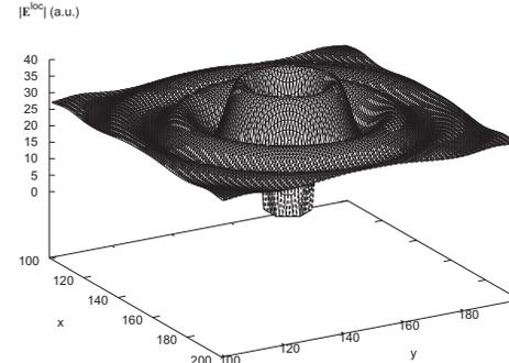
Fig. 2. The distribution of the local field  $E^{\text{loc}}$  in the vicinity of a circular hole in a planar triangular lattice of dipoles. Both  $E^{\text{ext}}$  and  $E^{\text{loc}}$  are perpendicular to the plane of the lattice. The distances along the  $x$ - and  $y$ -axes are normalized to the spatial period of the lattice.
